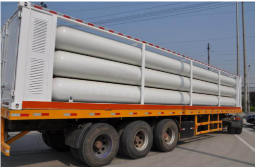
Trucking Raw Biogas to centralized processing plant
